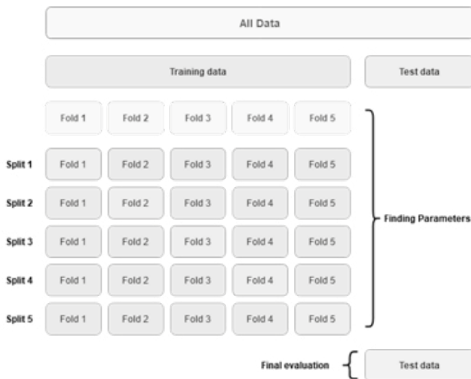
Figure 4. The performance measure by k-fold cross-validation
